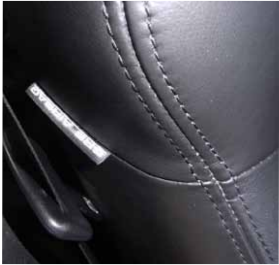
Seat Stitching for Air Bag Deployment
