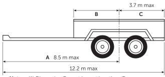
Note (1) Dimension B must be not less than C
