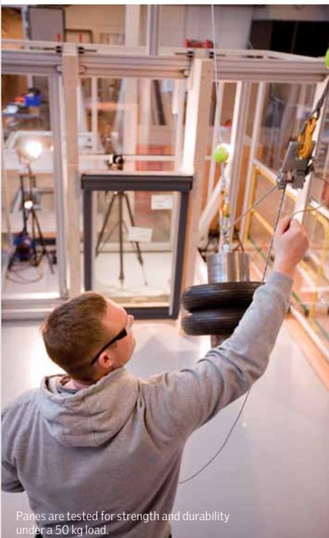
Panes are tested for strength and durability under a 50 kg load.
