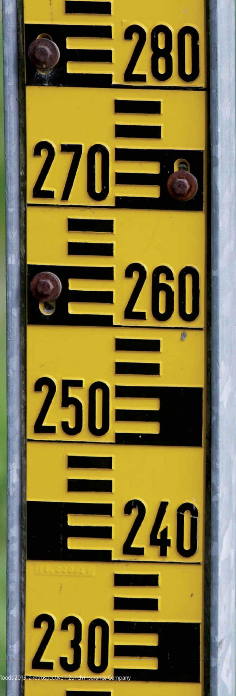
A flood gauge in Landshut's 'Flutmulde.' Normally on dry land, when floods rise to a certain level on the gauge, water is diverted out of the Isar.
