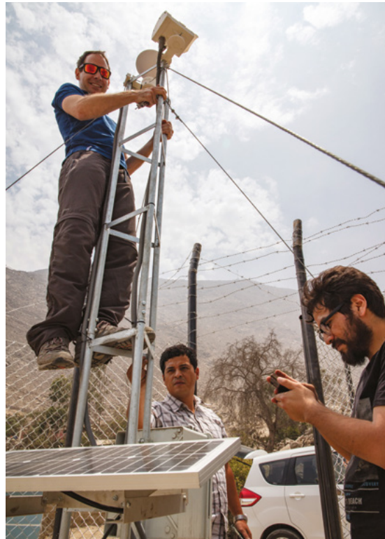
Michael Szönyi, Zurich's flood resilience program lead, tends to a warning system camera, while Miguel Arestegui of Practical Action, who developed the simple, cost-effective technology, checks the camera image on his smartphone. Photo: Emilie Etienne
