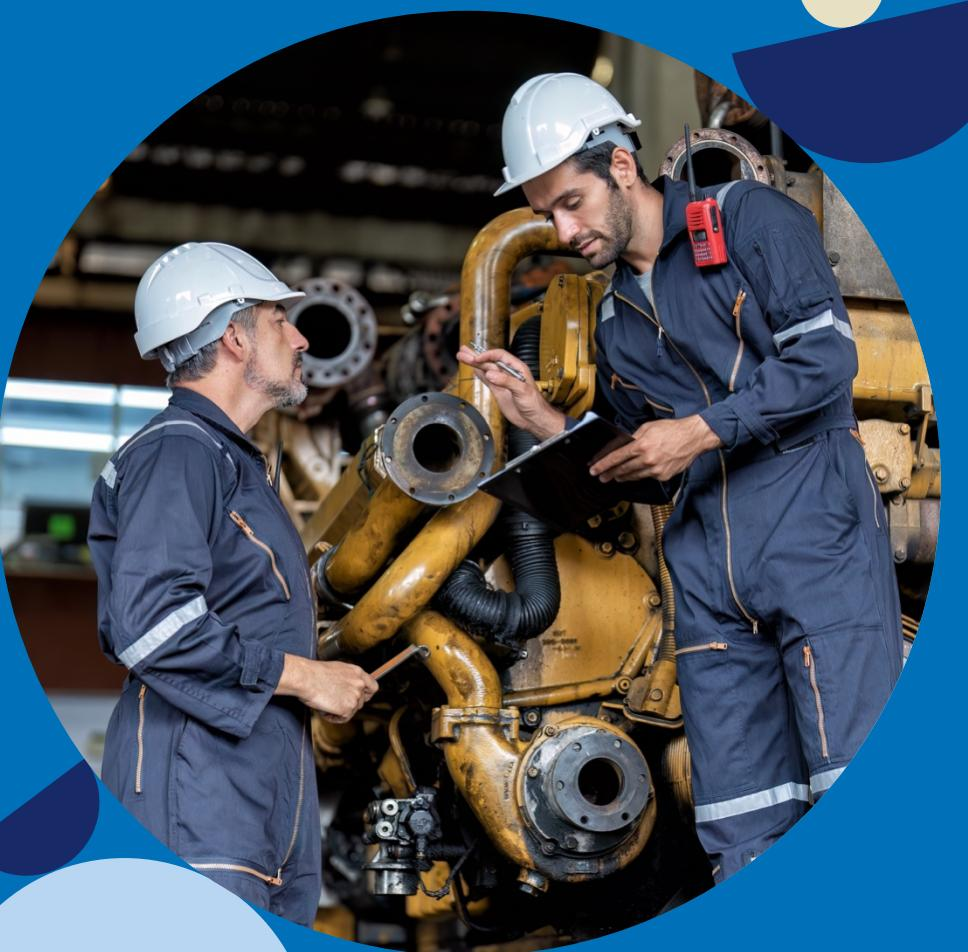
Diesel engines make up the vast majority of prime movers for emergency power generators due to their reliability, durability, and performance under load.
