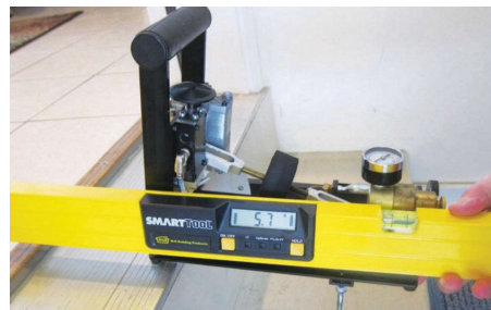
Proper set up of English XL VIT being evaluated before testing of a stair nosing begins.
