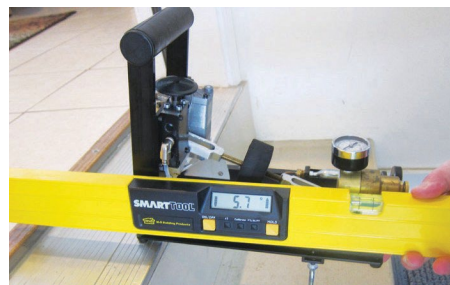
Proper set up of English XL VIT being evaluated before testing of a stair nosing begins.
