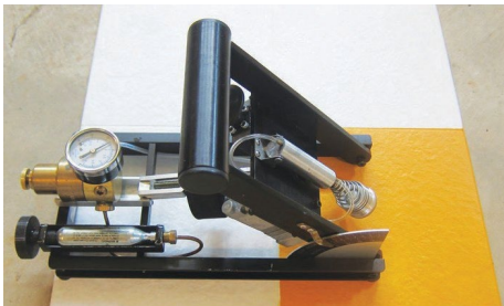
Testing of six paint samples showed that a flat latex paint provided the most slip resistance, followed by yellow parking lot marking paint.
